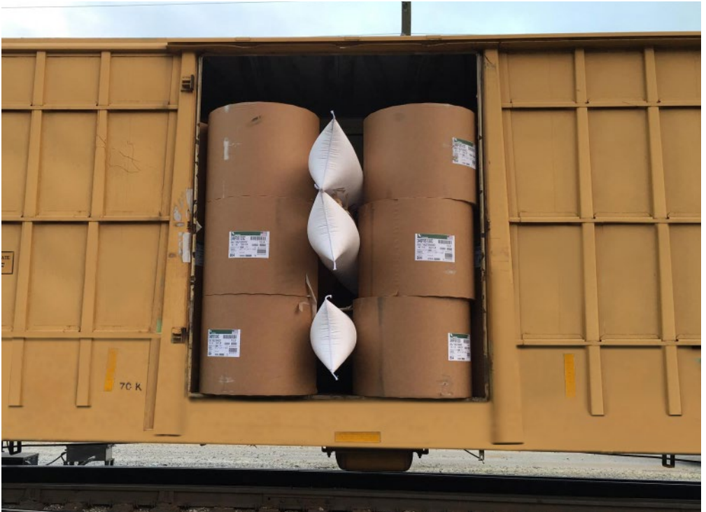
An example of doors that have been left open
